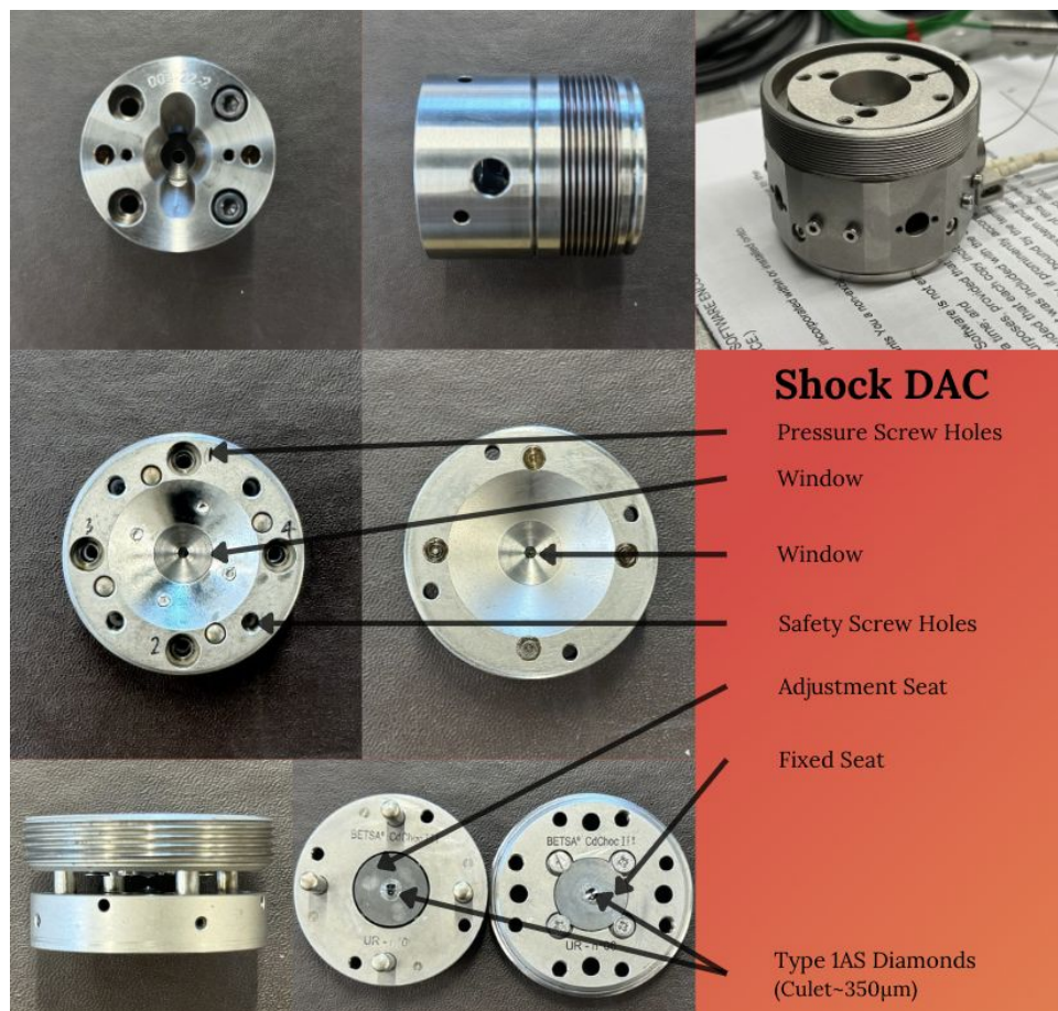
Figure 3. Different types and Components of a DAC
